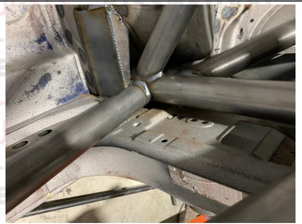
PHOTO 4 MAIN ROLLBAR TO FLOOR ATTACHMENT
