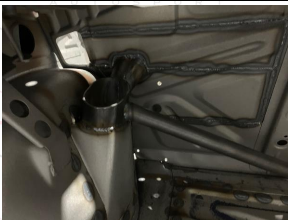
PHOTO 5 REAR BACKSTAY TO BODYSHELL ATTACHMENT
