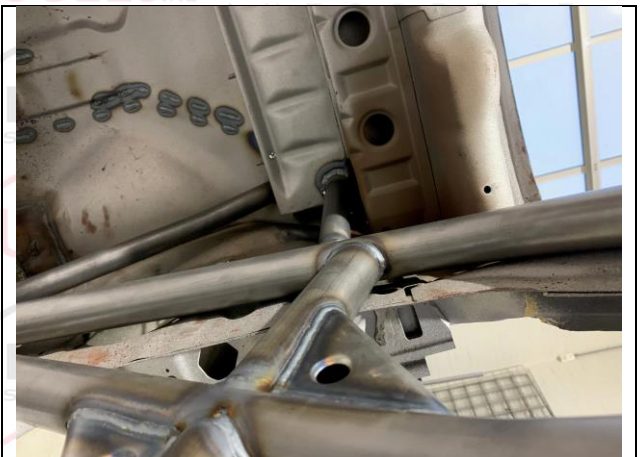
PHOTO 6 FRONT ROLLBAR TO FLOOR ATTACHMENT
